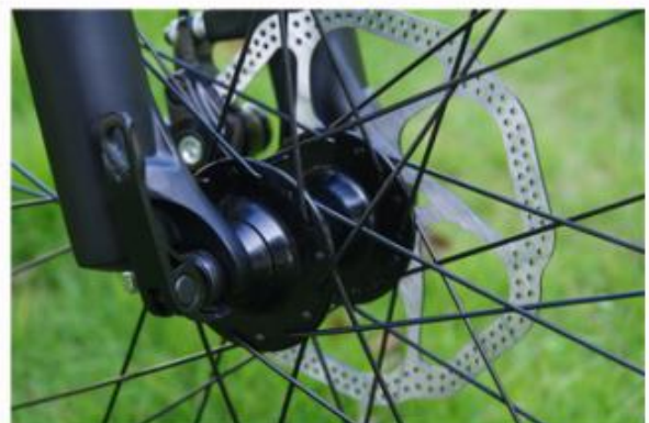
Front alloy hub with quick release axle
