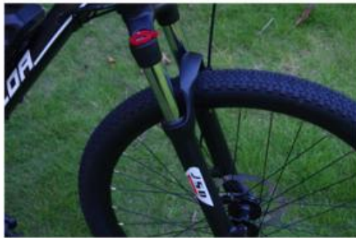
Front suspension fork with lockout
