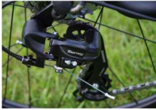
Shimano 24 speed gears(front 3*rear 8)
