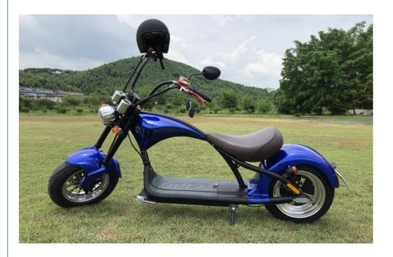
FrameSeamless steel pipeMotor1500-2000WBattery60V 12-20Ah lithium batteryController60V intelligent controller
